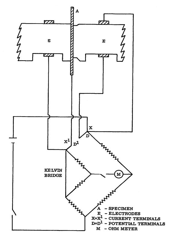
FIGURE 2. Circuit diagram for contact resistance measurements.
