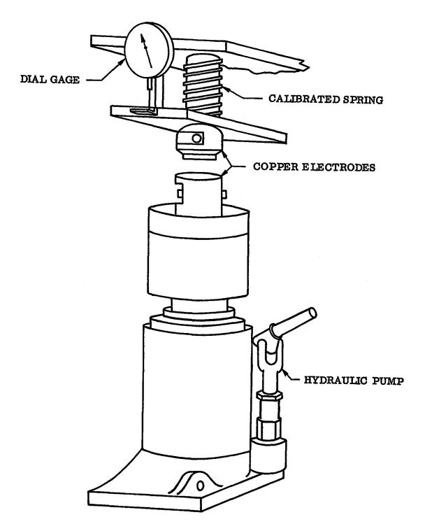
FIGURE 1. Sketch of equipment for measuring electrical resistance of chemical film.
